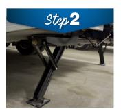
**TO EXTEND:** Press the "EXT" buttons until each arm reaches the ground. The sound of the motor will change pitch as the arms begin to take weight. Adjust each side independently for desired stability.
