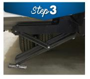
**TO RETRACT:** Press the "RET" buttons simultaneously until each arm is fully retracted.
