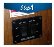
Use the extend and retract buttons in the coach to extend or retract the stabilizer arms. The arms operate and are controlled independently of one another.
